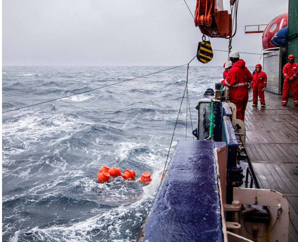
Researchers on the Polarstern icebreaker recover a sediment trap from deep waters in the Weddell Sea, Antarctica, as part of a project to understand more about the ocean as a long-term carbon sink (Image: Izzet Noyan Yilmaz / Alamy)
