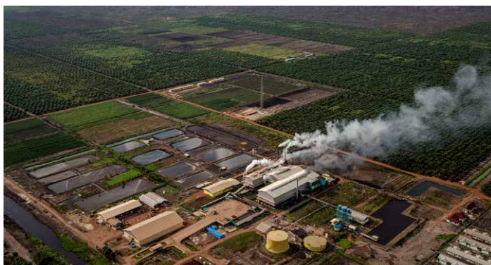
Fields of crops surround a palm oil mill in Central Kalimantan, Indonesia. To the left are ponds of oily wastewater which emit methane. (Image © Ulet Ifansasti / Greenpeace)
