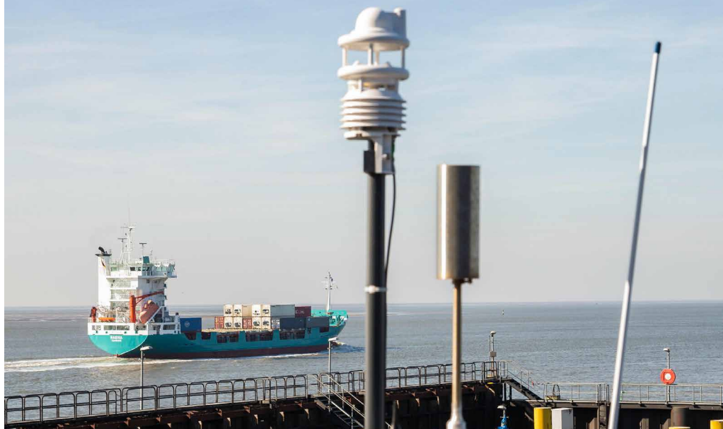
A container ship by a station near Bremen, Germany, for measuring the sulphur emissions of vessels passing in the North Sea (Image: Mohssen Assanimoghaddam / Alamy)
